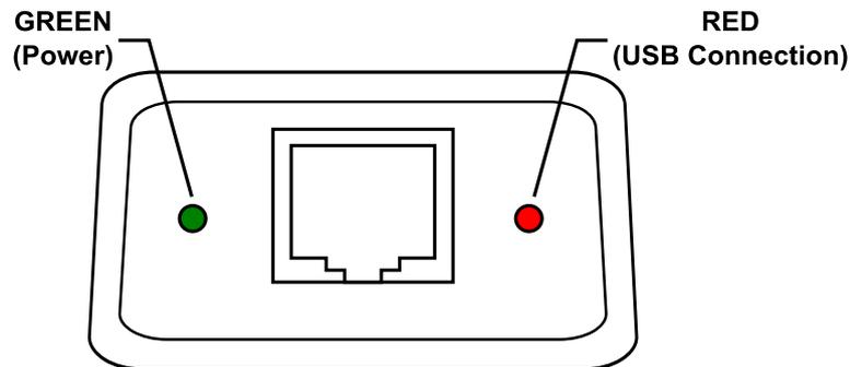
1. Green led - connection with AC/DC power adapter
